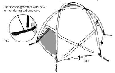
**5.** Slide three remaining poles into the color coded lower set of sleeves. Make sure that each pole passes though one color only. Take care, as you slide the pole, to follow the curve of the tent. Insert a pole end tip into the second grommet on each web. See fig.5.
